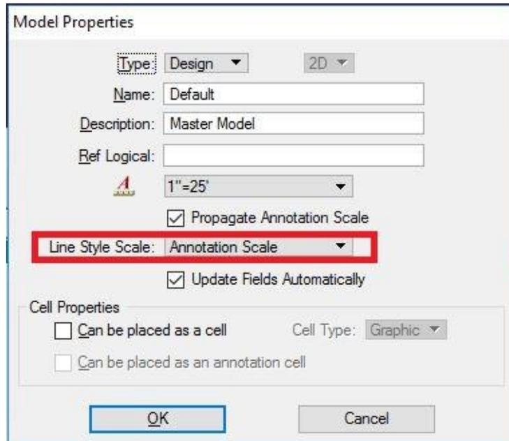
2. Please be sure the drawing scale in the file is set to either 1"=25' or 1"=50'. The line styles will not display correctly if the scale is set to Full Size 1=1
