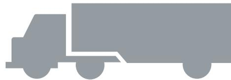
A **Multi-Unit Vehicle** is any combination of tractor and trailer that can be easily separated. These vehicles are also sometimes referred to as truck-tractor, semitrailers or combination vehicles.
